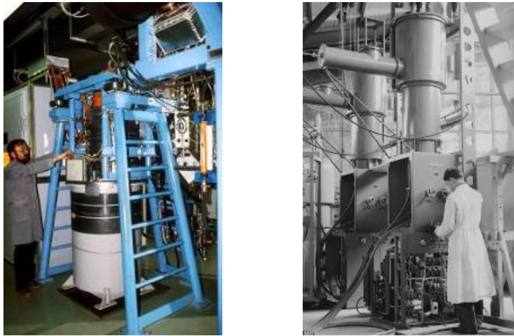
Fig. 20: A 3 GHz klystron amplifier for the LPI electron linac (left) and a 200 MHz triode-based amplifier for the Linac3 ion linac (right), both used at CERN
