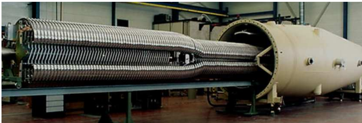
Fig. 12: Photo of 5 MV Tandatron in service position from HVEE (courtesy of H. van Oosterhout, HVEE)
