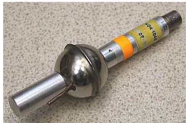
Figure 1. Hydrogen proportional detector of NOK-445 type.
