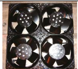
6.7 – Four fans used to blow cool air into enclosure (bottom side)
