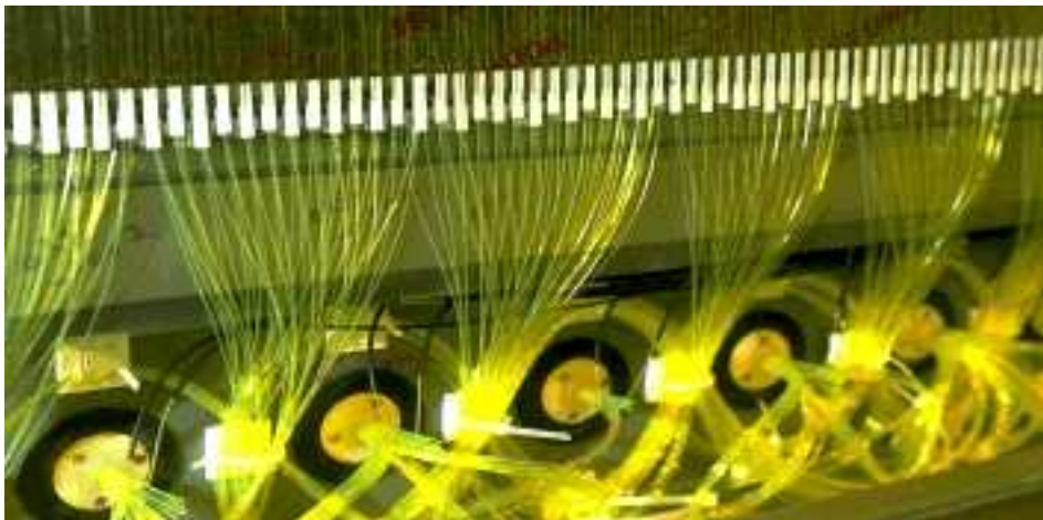
Figure 49: Picture of the optic WLS fibers bundles in a TileCal module connected to the PMTs for their read-out.
