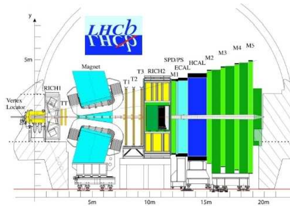
Figure 5: Scheme of the LHCb experiment for the LHC.
