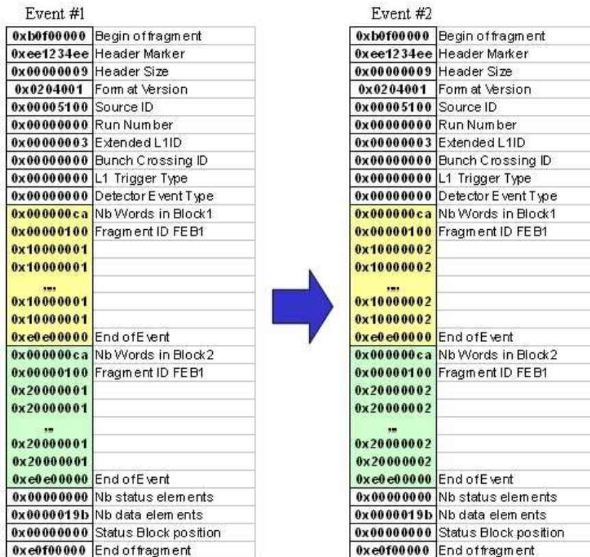
Figure 90: Scheme of the data format used for ROD pre-production tests. The two blocks of data with each FEB fiber output are coloured in yellow and green, respectively.
