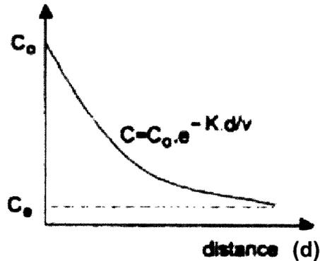
**Figure 4.3** Concentration profile for first-order decay in an ideal plug flow reactor (von Sperling, 2007).
