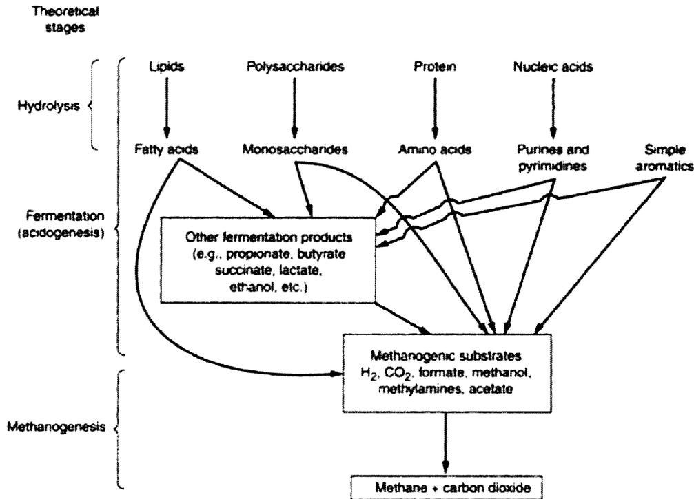
Figure 5.5 Schematic diagram showing the main stages in anaerobic digestion (Metcalf & Eddy, 2003).
