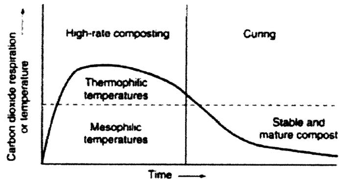
**Figure 5.6 Phases of the composting process with respect to carbon dioxide respiration and temperature (Metcalf and Eddy, 2003).**
