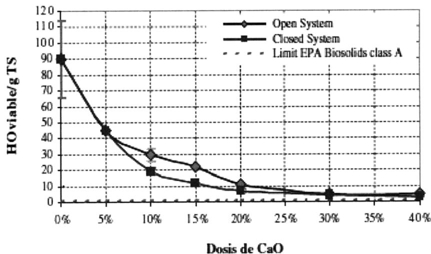
Figure 5.4 Inactivation of viable helminth ova (HO) in open and closed alkaline stabilization systems for various lime doses (Mendez et al., 2002).
