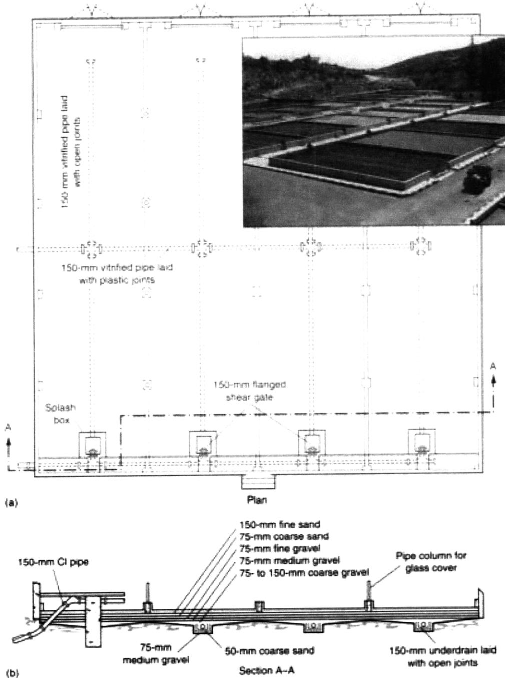
Figure 5.1 (a) Plan and (b) sectional view of a typical conventional sand drying bed. Top right image shows sludge drying beds containing sludges of different degrees of dryness (Metcalf & Eddy, 2003).
