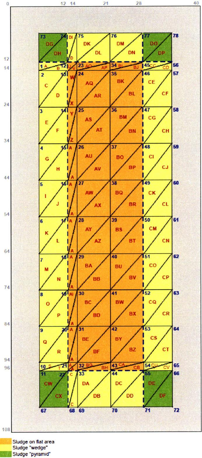
Puerto Cortes Anaerobic Lagoon 1: Node Coordinates
