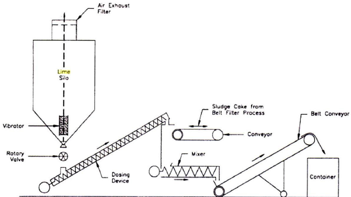
**Figure 5.2 Schematic of dry lime stabilization process**
