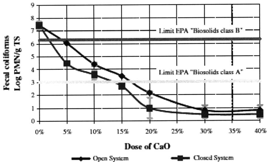
Figure 5.3 Inactivation of fecal coliforms in open and closed alkaline stabilization systems for various lime doses (Mendez et al., 2002).
