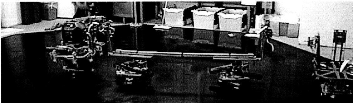
Figure 1.4: The SWARM propulsion module maneuvers a flexible beam element toward a fixed target on the right.
