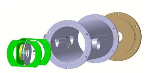
Fig.3-A1: Integration of the mirror support inside the end-cap.
