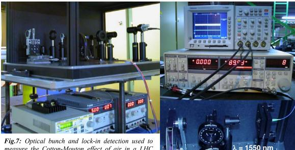
**Fig.7:** Optical bunch and lock-in detection used to measure the Cotton-Mouton effect of air in a LHC superconducting dipole. For the double paths of the laser beam inside the magnet aperture, a mirror was positioned outside at one of the magnet extremities.
