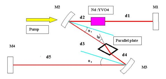
**Fig. 10:** Schematic diagram of a Z-fold cavity of the Nd:  $YVO_4$  laser. The Nd:  $YVO_4$  crystal is the laser gain medium whereas the Brewster plate is used to polarize the light beam.
