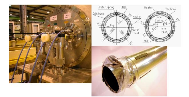
Fig.1-A1: Anticryostats mounted inside a LHC cryodipole
