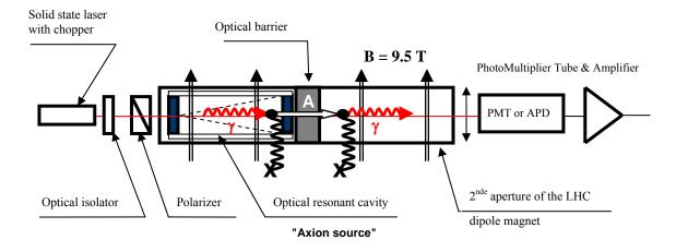
Fig. 9: Principle of the photon regeneration experiment.
