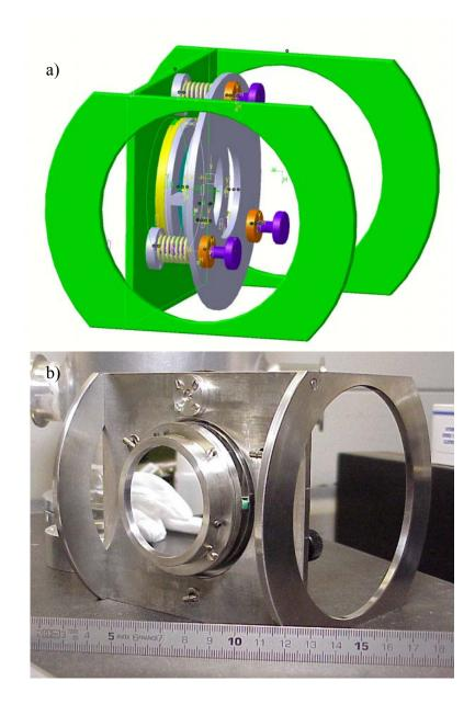
Fig.4-A1: Mirror support a) drawing, b) first prototype
