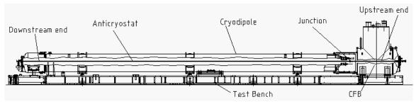
*Fig. 5:* Layout of a cold test bench for dipole magnets equipped with anticryostats and connected to its Cryogenic Feed Box (CFB). The overall length is equal to 19.6 m.
