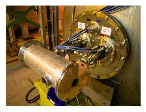
Fig.2-A1: Prototype end-caps connected to the Anticryostats
