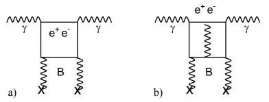
**Fig. 1:** Feynman diagrams for light-by-light scattering producing the magnetic birefringence of the vacuum due to the photon dispersion; a) the dominant term and b) one of the second order diagrams with radiative correction.
