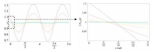
**Fig.2-A2:** The ratio  $2P_{4\omega}/\beta$  as a function of  $\gamma$  for  $\delta = \varepsilon = 5.10^{-4}$ ,  $\delta\theta = 10^{-4}$  and  $\delta\chi = 3.10^{-4}$ . The plots with decreasing maximums correspond to the values of  $\beta = 10^{-7}$ ,  $2.10^{-7}$ ,  $5.10^{-7}$ ,  $10^{-6}$ ,  $5.10^{-6}$ ,  $5.10^{-6}$  and  $> 10^{-5}$  respectively.
