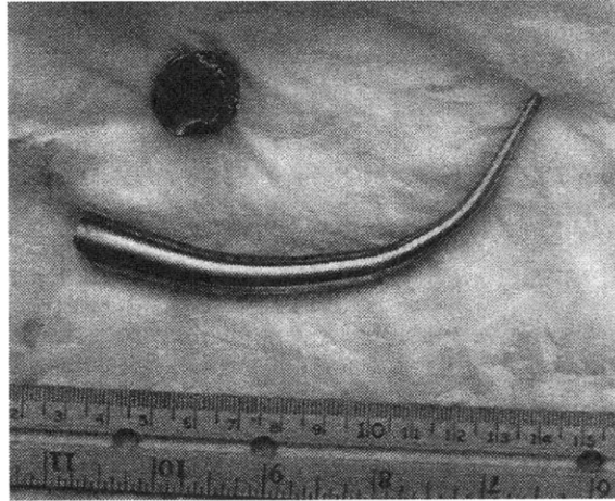
Figure 6-3: Projectile bent during underwater testing of supercavitating bullets [6].
