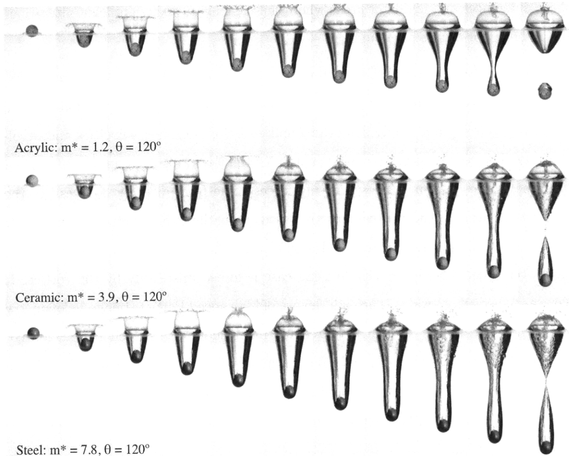
Figure 3-1: Three different spheres of the same diameter ( D = 0.0254 m) dropped from the same height ( h = 60 cm), coated with the same surface treatment (advancing contact angle \theta = 120^\circ ) but all have different mass ratios m^* = \rho_s/\rho as indicated. The time between images is 7.1 ms and the impact speed is V_i = 3.43 ms -1 yielding the same Froude number F = V_i/\sqrt{gD} = 6.87 for all cases.
