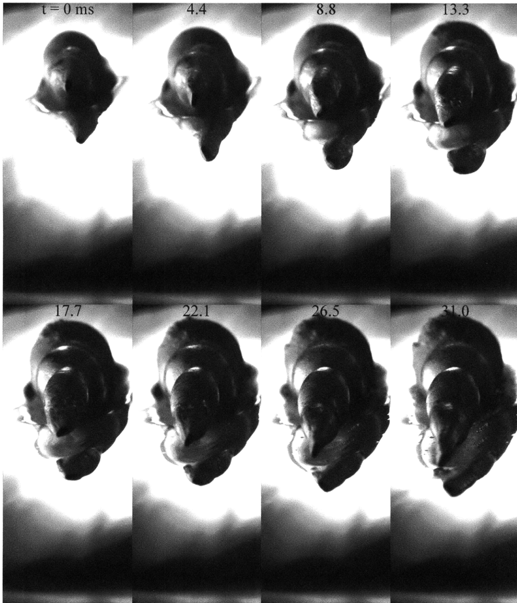
Figure 8-10: Images of a modified 22 caliber aluminum bullet case number (1,14,2) viewed looking at bullet head on. This bullet type corresponds to bullet name #1 was fired at 1250 ft/s from the rifle barrel at an angle of 10.7^\circ (see table 8.2. The camera acquired images at 2260 f/s, and every image in series is presented here.
