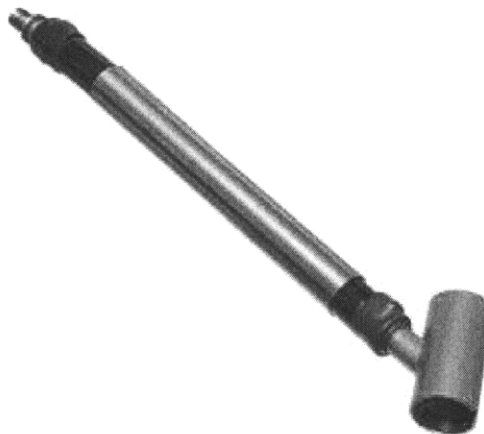
Figure 6.18 Modified Golf Pro with a titanium tube over the flexible coupling
