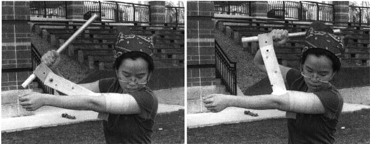
Figure 8.5 (a) Right arm pulling the prototype straight and (b) Right arm pulling the prototype around the head and the prototype bending at the elbow joint
