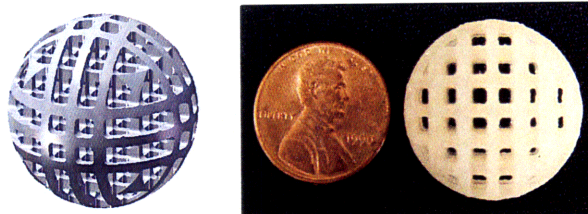
Figure 2.44: 3D sphere design used to demonstrate anisotropic stiffness.
