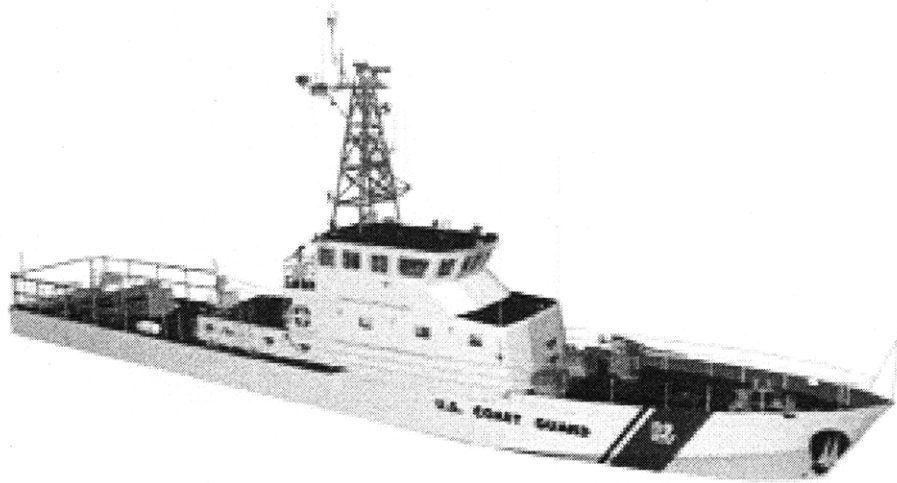
Figure 4: A CAD rendition of the United States Coast Guard 123' Patrol Craft. This Cutter was first built as a 110' Patrol Boat and retrofit with a stern launch as part of the Deepwater Program.
