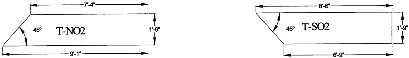
Figure 8.41 Top view of spacer blocks T-NO2 and T-SO2. T-NO2 is located on top of the outer right side wall. T-SO2 is located on top of the outer left side wall.
