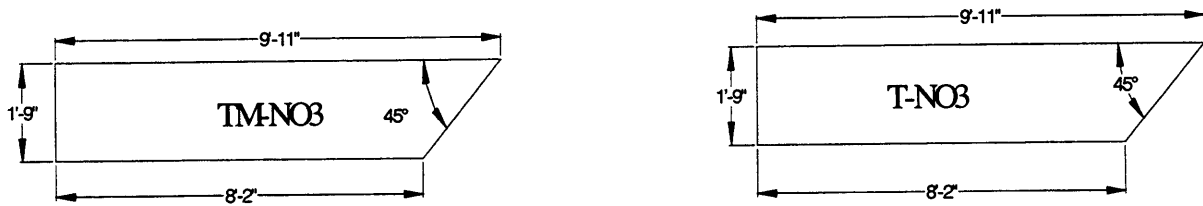
Figure 8.46 Side view of spacer blocks beneath the “blocks next to shutter”. These blocks will hold the inlet into the exhaust ventilation ducts.
