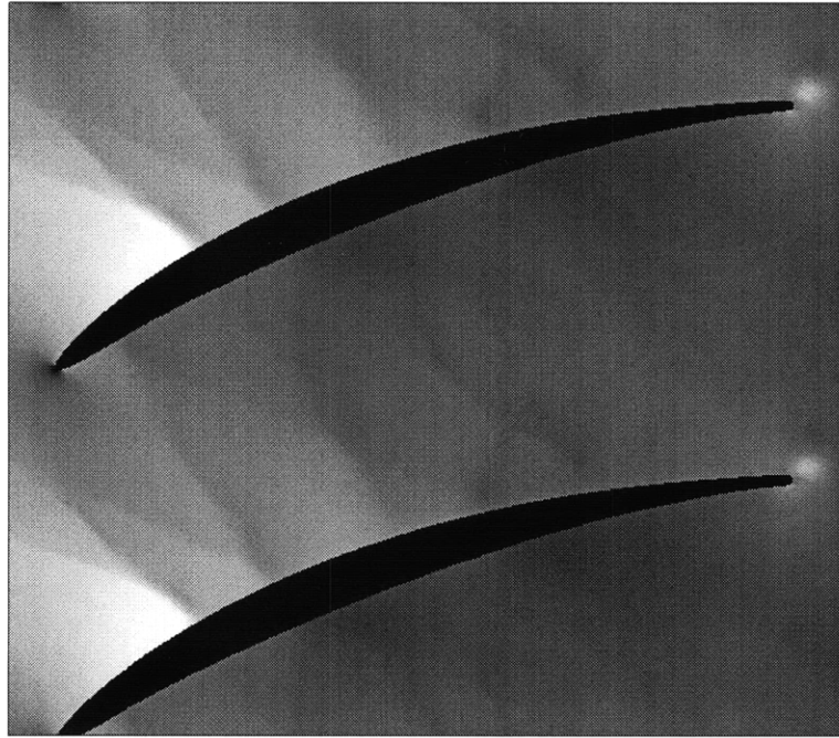
Figure 3-14: Pressure contours of the baseline solution for Run 4. The pressure waves can be seen as dark lines extending across the blade passage. M_\infty = 0.87 . Re(c, U_\infty) = 0.8 \times 10^6 .
