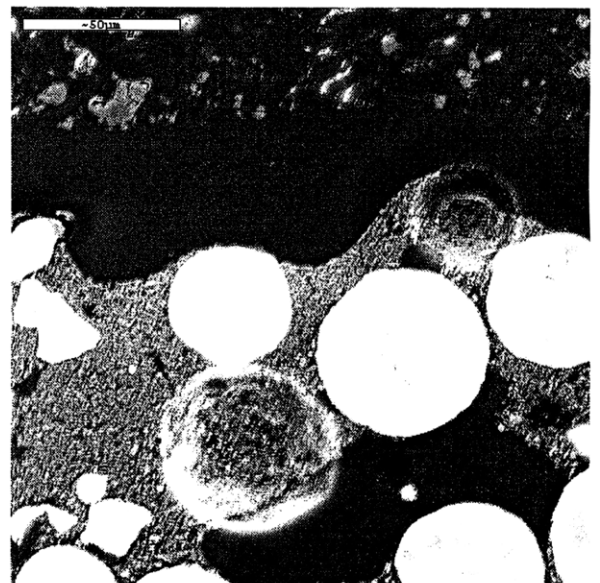
Figure 4.16 e) 5 mil, Single Printed Molybdenum-TiC Section; 200 micron scale bar. f) Top Surface of 5 mil, Single Printed Molybdenum-TiC Section; 50 micron scale bar. (All samples printed at 170 micron line spacing)
