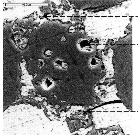
b) TiC infiltrated with Cu-Ni-Mn, 20 micron scale bar.
