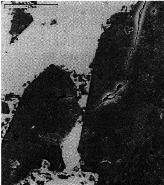
Figure 4.6a) 74-105 micron & Sub-micron TiC; 73.5:26.5, Large to small powder concentration ratio (20 micron scale bar).
