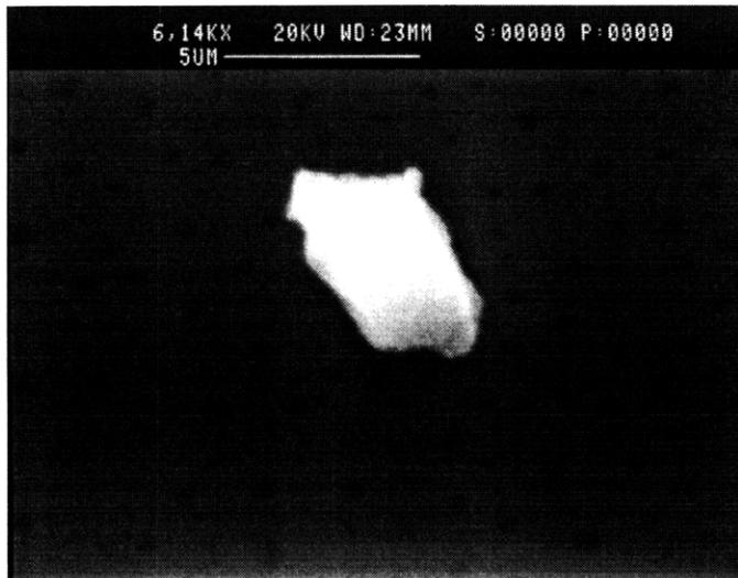
Figure 19: SEM micrograph of anodized aluminum (magnification of Figure 18)
