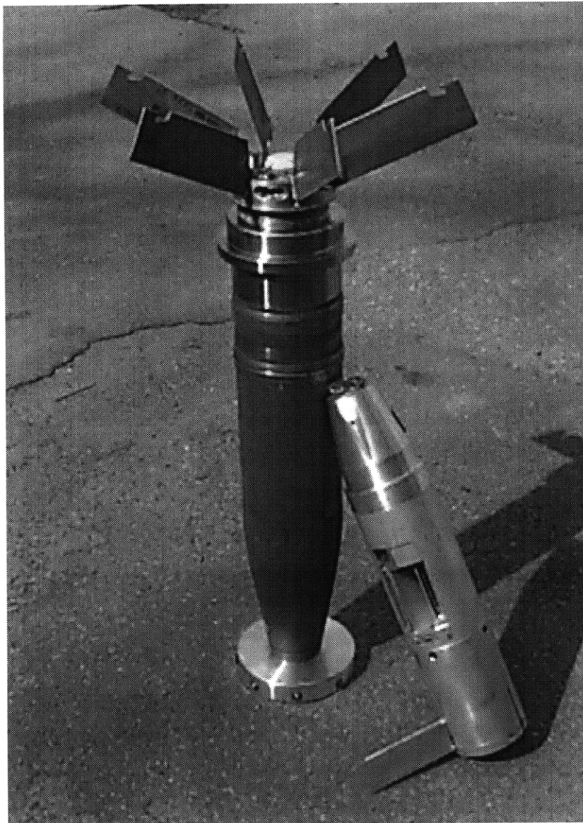
Figure 9: Shell with Six Fins Deployed and Flyer
