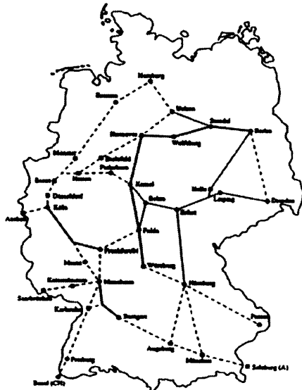
Fig. 4. German high-speed rail routes for the year 2010 ——— Neubaustrecke in service or confirmed, - - - - - Additional "Unification" routes studied, . . . . . Other NBS/ABS routes
