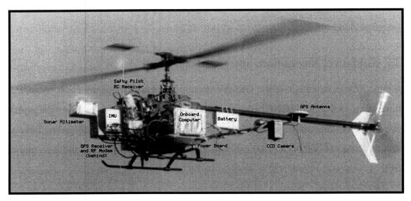
Figure 2.1: DSAAV in flight
