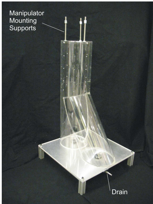
(a) Test tank with manipulator mounting supports affixed at top of main bore.
