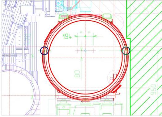
Figure 5: Cross-section of the cryostat, indicating where the BLMs will be positioned. The proposed location to install the BLMs is indicated by the solid black circles. The green hashed area to the right-hand side indicates the space reserved in the tunnel for transport.
