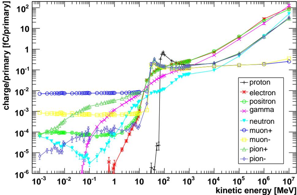
Figure 4: BLM response to different particle species as a function of incident energy of the particle. From [7].
