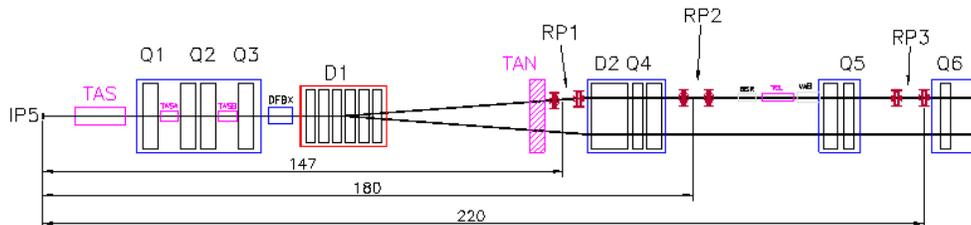
Figure 1: Machine Elements in LSS 5. RP1 indicates the location of the 150m station, and RP3 indicates the location of the 220m station. RP2 represents a possible station for TOTEM Roman Pots, which may be installed at a later stage.
