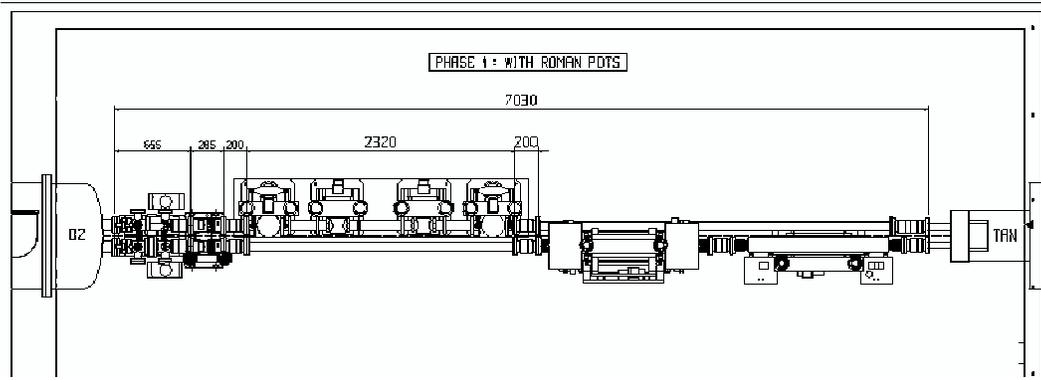
Figure 2: Drawing of the TOTEM 150m station showing the details of the integration between TAN and D2. From [6].
