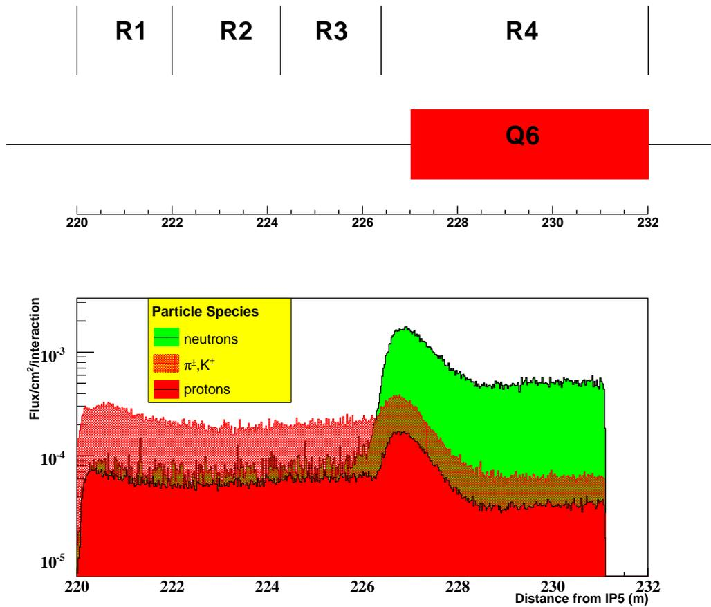
Figure 8: Particle flux density recorded across the scoring plane as a function of distance from IP5 for simulation of the 220m station. Charged pions and kaons are represented by the red line, protons by the red histogram, and neutrons by the green histogram. The regions of interest, defined later in the text, and the positions of the magnetic coils are indicated at the top of the figure.
