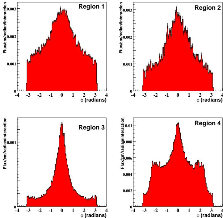
Figure 7:  $\phi$  dependance of particle flux for the simulation of the 150m station.  $\phi$ , in radians, is defined so that 0 corresponds to ring outwards,  $\pm\pi$  to ring inwards,  $\pi/2$  as up and  $-\pi/2$  down.
