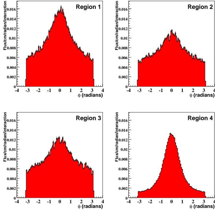
Figure 9:  $\phi$  dependance of particle flux for the simulation of the 220m station.  $\phi$ , in radians, is defined so that 0 corresponds to ring outwards,  $\pm\pi$  to ring inwards,  $\pi/2$  as up and  $-\pi/2$  down.
