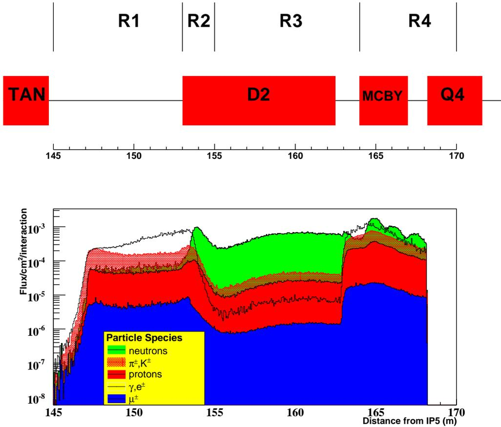
Figure 6: Particle flux density recorded across the scoring plane as a function of distance from IP5 for simulation of the 150m station. The particle species shown are: neutron (green histogram), proton flux (red histogram), muon flux (blue histogram), charged pion and kaon flux (red line), and the photon and electron flux (black line). The regions of interest, defined later in the text, and the positions of the magnetic coils are indicated at the top of the figure.
