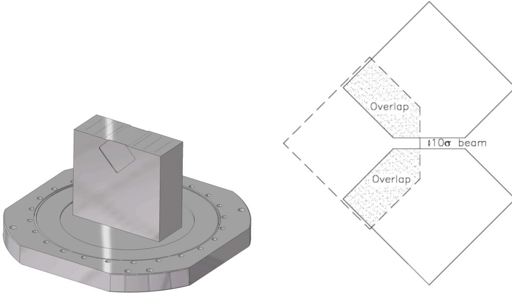
Figure 3: Geometry of Detector Pot to be inserted close to the beam (left). The detector configuration (right) consists of 2 vertical detectors (solid lines) at the same location in  $s$ , and 1 horizontal detector (dashed lines), offset by  $\sim 90\text{cm}$  in  $s$ .
