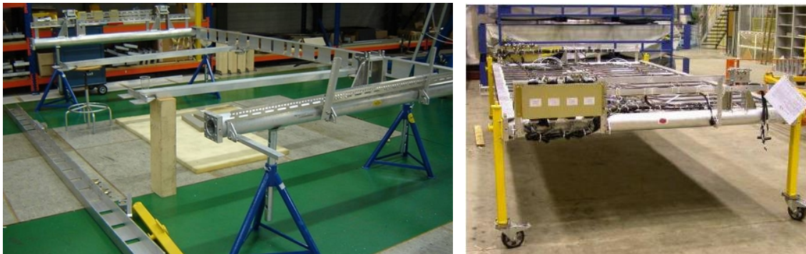
Figure 21: BOS common support – RPC package. Different from other chamber types the common support in the case of BOS completely surrounds the RPC in the form of a 'cradle'. The MDT chamber is added in a second step.
