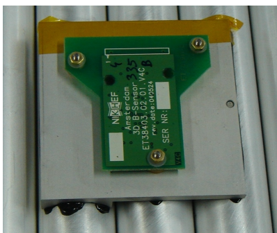
Figure 5: Magnetic field probes are mounted on special platforms glued onto the MDTs of BOS/F/G, BMS and certain BOL chambers.
