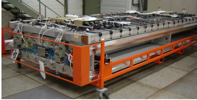
Figure 19: Assembled muon station of type BOL. Stations of type BO have one RPC plane only, with the exception of some BOF and BOG stations later located in the feet region of the experiment.
