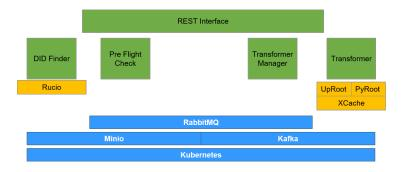
Figure 2. Architecture for ServiceX version 1.
