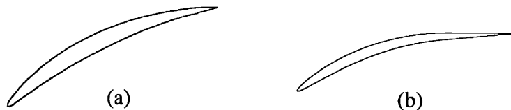
Figure 4.2: Blade geometries used for numerical experiments: EEE blade(a) with blade loading \psi \approx 0.5 and NACA4F blade(b) with \psi \approx 0.31 .
