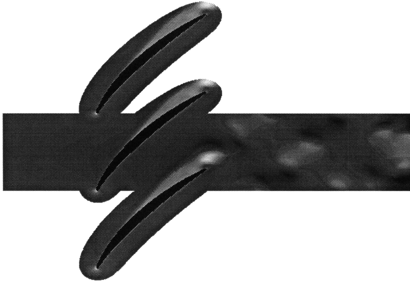
Figure 5.10: Axial velocity contours for steady state flow with Re = 1e6 .
