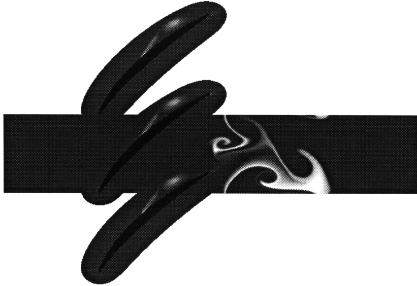
Figure 5.7: Constant density contours for wake leaving trailing edge with \rho^* = -\frac{1}{3} , \frac{w}{c} = 0.4 , and \text{Re} = 1e6 .
