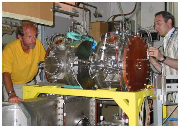
Figure 6: The CCDTL prototype (2 half-tanks with coupling cell) ready for high-power RF testing.
