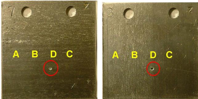
Figure 11: Zn-plates 7 and 8. The melting agrees with the simulation.
