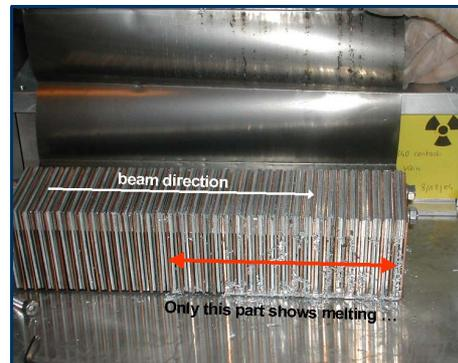
Figure 10: The core of the target after the test. On the more downstream part melted Zn can be seen.
