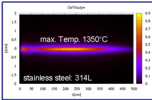
Figure 3: Results of one of the FLUKA simulations to reconstitute the observed energy deposition in the QTRF vacuum pipe.
