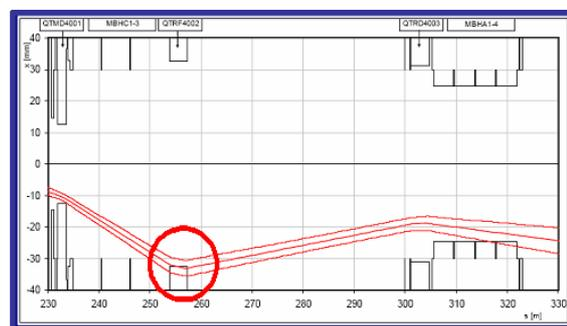
Figure 2: Reconstructed trajectory hitting the QTRF vacuum chamber during the TT40 accident.
