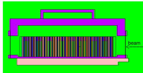
Figure 6: The model of the target implemented in FLUKA.
