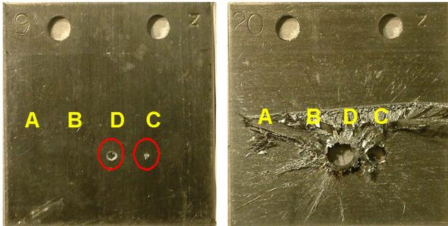
Figure 12: Zn-plates 9 and 20. Holes and melting agree with the simulation.
