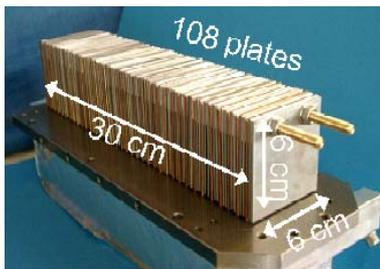
Figure 4: Core of the target for the damage test in TT40.
