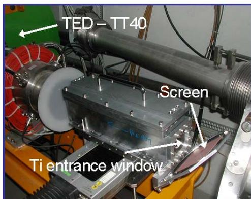
Figure 8: The target installed in TT40 in front of the TT40-TED in air.
