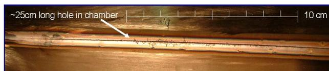
Figure 1: Damaged vacuum pipe of the QTRF pipe in TT40.
