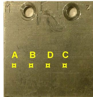
Figure 9: Plate 1 of Zn after the test. The locations of the four different intensities are indicated.
