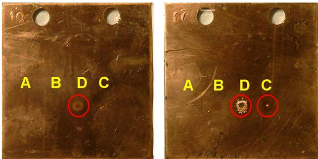
Figure 13: Cu plates 10 and 17. Prediction for plate 10: no melting. Observation: signs of heating, no melting. Prediction for plate 17: melting for D. Observation: melting for D and C. However, prediction for plate 18: melting for D and C. Agreement within 0.5cm.
