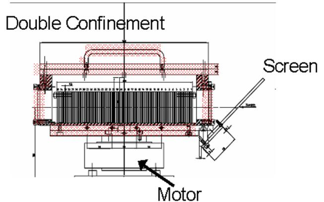
Figure 5: Target with outer confinement, motor and screen.
