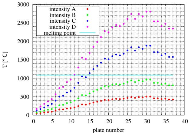
Figure 7: FLUKA results for the temperature in the Cu plates for the different intensities. Heat of fusion is not taken into account for this graph.
