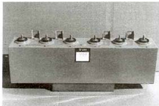
Fig. 14: Filter capacitor for an IGBT traction converter (tramway). Segmented metallized rape-oil impregnated polypropylene technology. The 3 element with flat terminals give this capacitor a series inductance < 30 \text{ nH} (3150 \mu\text{F} , 1000 V, 690 \times 140 \times 185 \text{ mm}^3 ).
