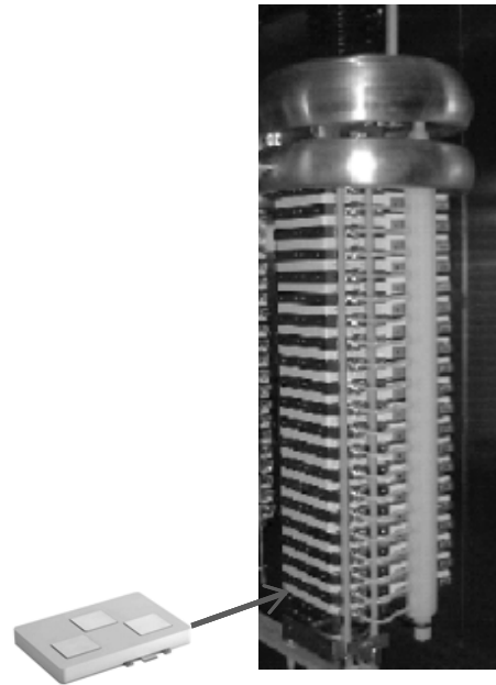
Fig. 7: An HVDC valve for a VSI. Each valve contains 20 IGBT press-packs and many valves may be series connected for a typical high-voltage DC transmission system.
