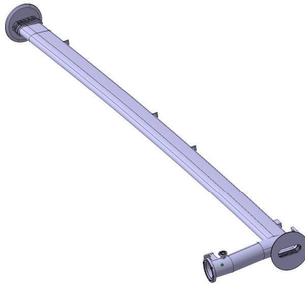
Fig. 47: Layout of the new vacuum chambers for magnet units 14 and 15
