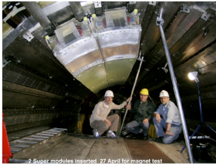
Figure 12. First two ECAL SM inserted into the HCAL for the Cosmic Challenge.
