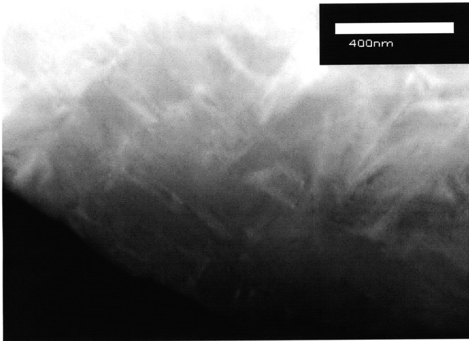
Figure 6.3 Bright field STEM micrograph of cross-section TEM sample of SA2 before oxidation. The region of the sample investigated is approximately 100-200 \mu\text{m} below the polished surface.
