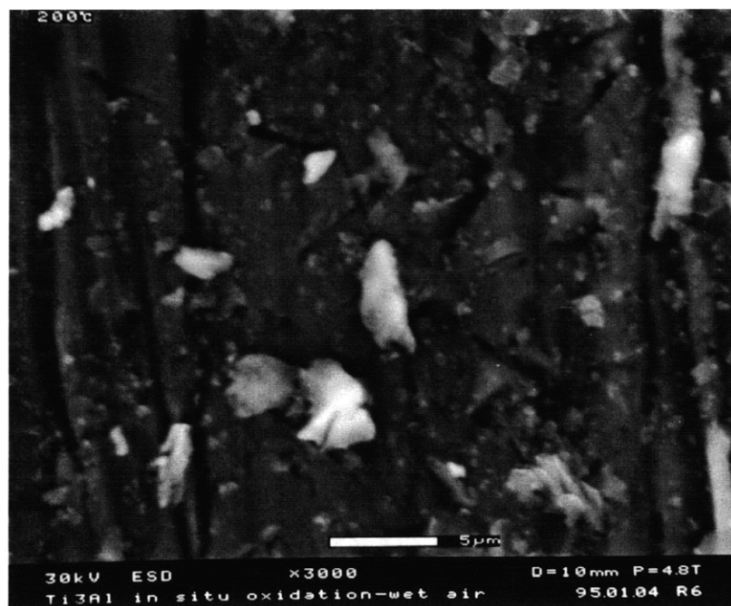
Figure 7.1 ESEM micrograph of Alloy A2 oxidized in-situ in moist air showing small oxide nodules nucleated at approximately 200°C.
