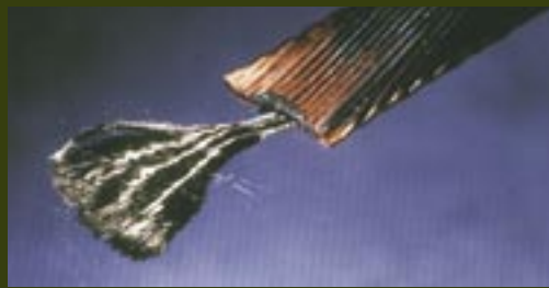
Left: Superconducting cables form the heart of the LHC's particle colliding ability. Each cable consists of 6000 coated superconducting wires. Manufacturing the cables took a joint effort between CERN and industry.
