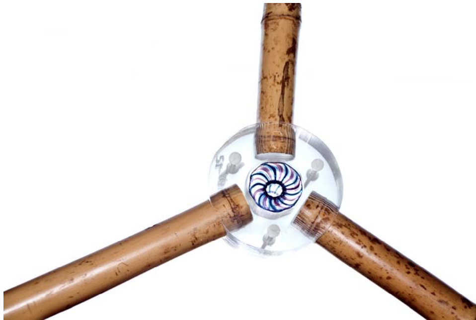
Figure 31: The Bamboo-Glass Joint
