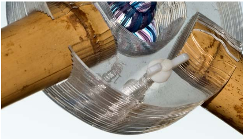
Figure 33: Smaller Error in the Layered Joint after Measuring (Sensing) Layer Thickness
