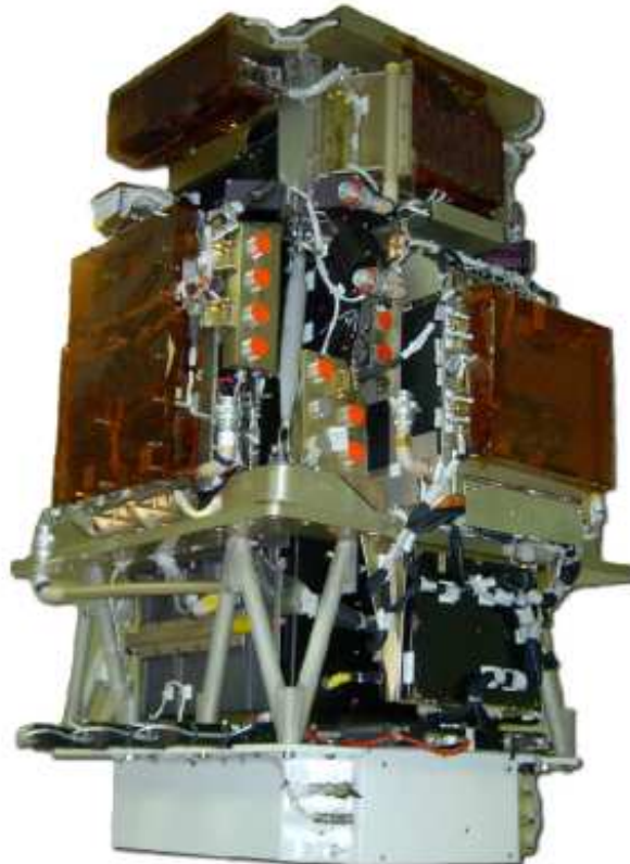
Fig. 4. The PAMELA instrument. Top: a schematic overview of the apparatus. Bottom: a photograph taken just prior delivery to Russia for integration with the Resurs DK1 satellite. The detector is approximately 1.3 m tall. The magnetic field lines in the spectrometer are oriented along the y direction.
