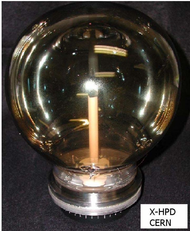
Fig. 2: Photograph of the X-HPD prototype with 208 mm diameter glass envelope.
