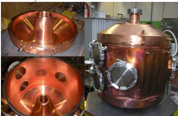
Fig. 3: 200 MHz capture cavity (right) and parts of it before brazing (left).
