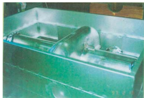
Figure 36: Annealing at 700°C for 3 hours of KEKB crab cavity [33].
