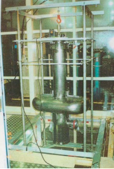
Figure 37: High-pressure water rinsing by 80-bar ultra-pure water of KEKB crab cavity [33].
