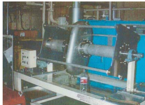
Figure 35: Barrel polishing of KEKB crab cavity [33].
