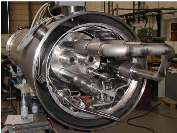
Figure 1: Quadrupole cold mass in cryostat, prepared for cold tests.
