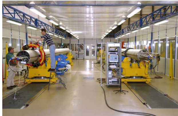
Figure 3: Closure and geometrical verification of the quadrupoles are performed on two alignment benches.
