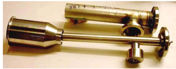
Figure 4: Welding tooling used to minimise deformation.
