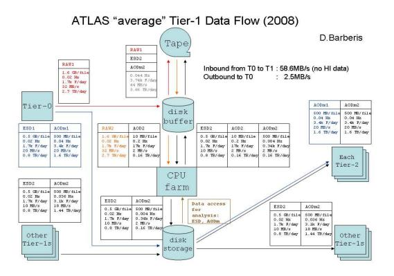
Figure 1: ATLAS "average" Tier-1 data flow (without MC data)
