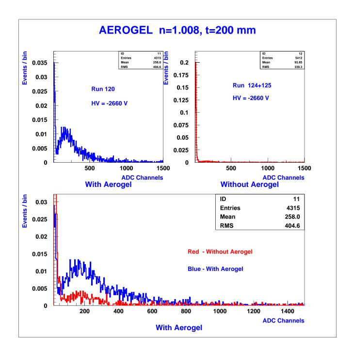
Figure 4: ADC-spectra for the Aerogel radiator with the refractive index of n = 1.008
