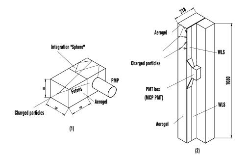
Figure 1: Classical TAC detector design – Belle Integration Sphere Type (1) and TAC detector design of ASHIPH type (2)
