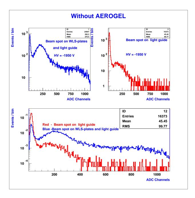
Figure 6: ADC-spectra for the radiator "without Aerogel"
