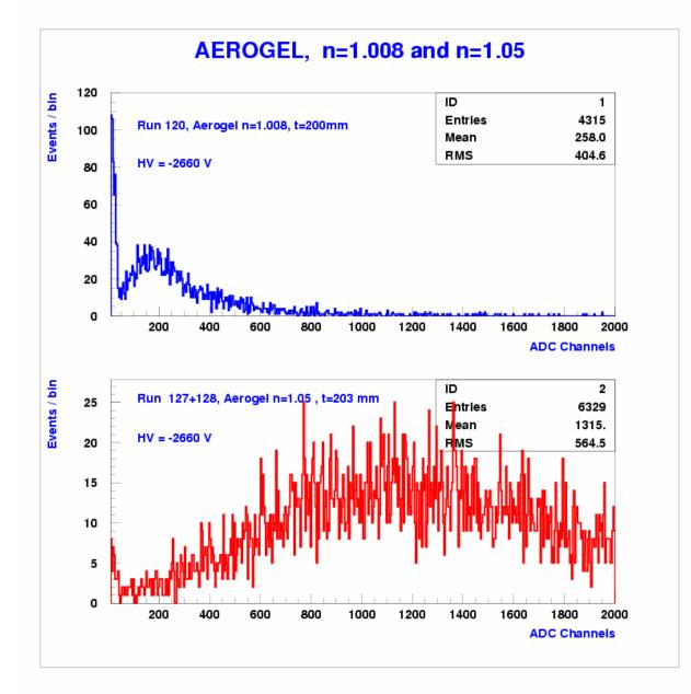
Figure 5: ADC-spectra for the Aerogel radiators with n = 1.05 and 1.008
