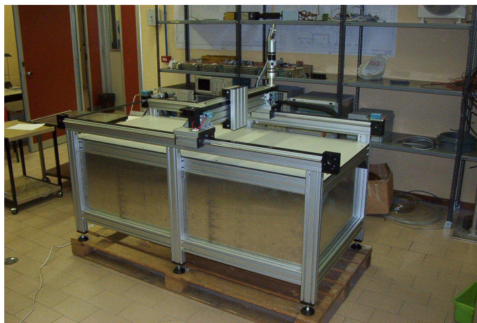
Figure 3.1: A photograph of the Rome2 system for gas gain measurements.
