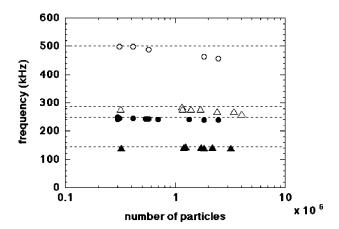
FIG. 4. The resonance frequency for the radial compression of protons (solid circles) and  $H_3^+$  ions (solid triangles) as a function of the particle number. Open circles and open triangles correspond to the second harmonic frequencies for the radial compression of protons and  $H_3^+$  ions, respectively. Solid circles are almost independent of the number of protons.
