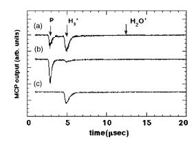
FIG. 2. Time-of-flight spectra of extracted ions with extraction energy of  $\approx 800 \text{ eV}$ . (a) Two peaks corresponding to protons and  $H_3^+$  ions are clearly observed. (b) rf field with a frequency of 142 kHz (axial harmonic oscillation for  $H_3^+$  ions) was applied to kick out  $H_3^+$  ions. (c) rf field with a frequency of 248 kHz (axial harmonic oscillation for protons) was applied to kick out protons.
