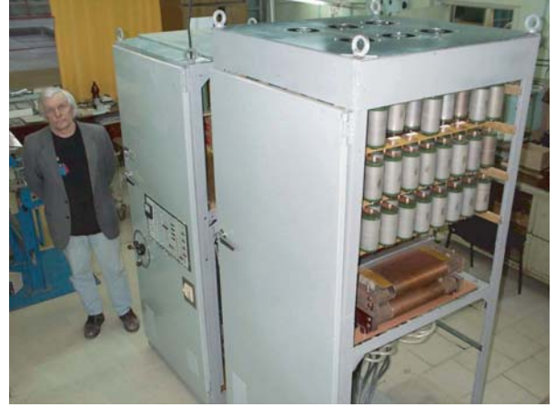
Figure 29: BINP modulator for the VEPP-5 positron flux concentrator developed by A.D. Chernikian [36].
