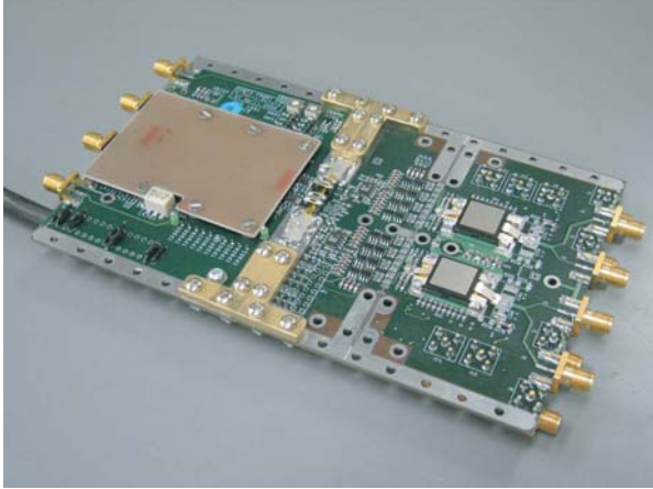
Figure 19: FONT3 printed-circuit-board amplifier and feedback [14].
