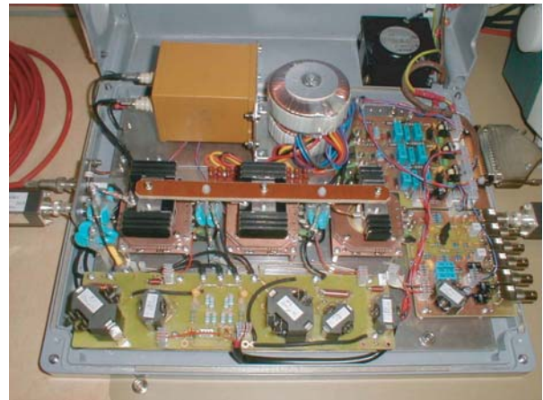
Figure 17: Components of FONT1 3-stage tube amplifier [14].
