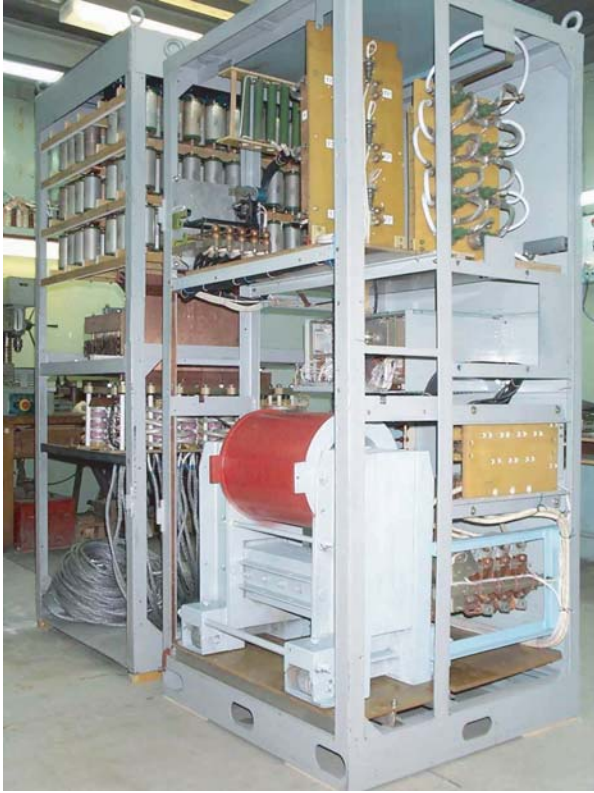
Figure 30: BINP modulator for the VEPP-5 positron flux concentrator developed by A.D. Chernikian [36].
