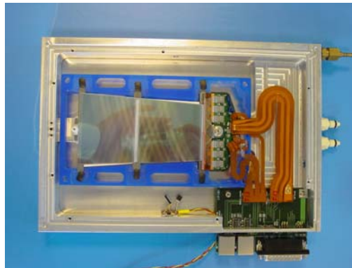
Figure 5.9. Photo of an outer end-cap module supported by its transport frame inside its aluminium test box. The dry-air and coolant inlets are visible, as well as the support card.
