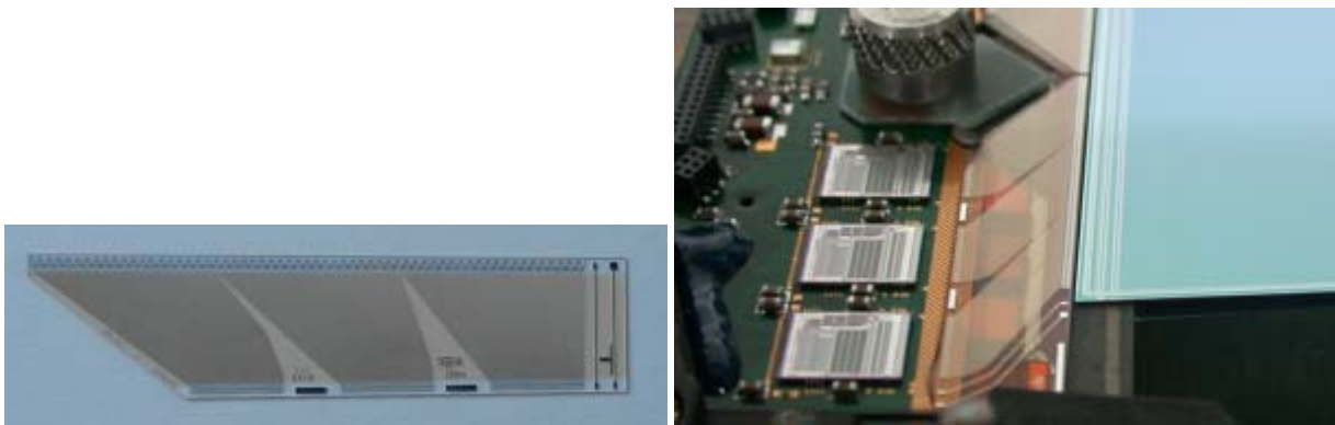
Figure 4.8. Left. A fan-in showing the traces from the ASICs (bottom) to the sensors (top). Right. Fan-in glued to the hybrid and the spine spacers.
