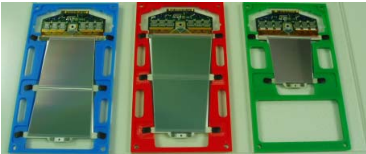
Figure 1.2. ATLAS SCT end-cap modules. From left to right: outer, middle and inner. There is a fourth type, the short-middle, that follows the design of a middle module with only a pair of silicon sensors.
