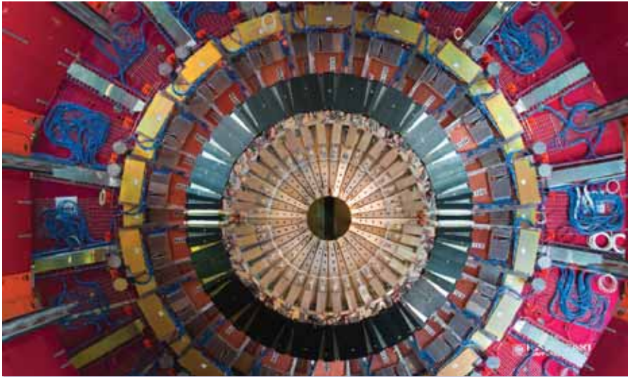
The concentric structure of the CMS detector is clearly visible during its assembly. When the LHC is running protons will collide head on at the centre, and the various layers will measure different particle properties, building up a complete picture of each collision recorded.
