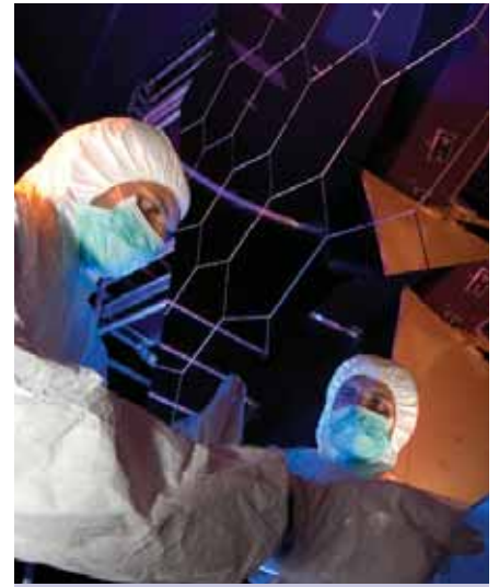
Assembly of a ring-imaging Cherenkov detector for the LHCb detector is carried out under extremely clean conditions.
