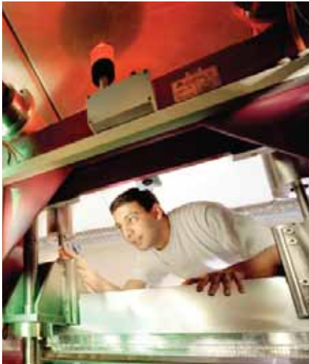
Undulators like this one at the European Synchrotron Radiation Facility shake photons from electron beams.
