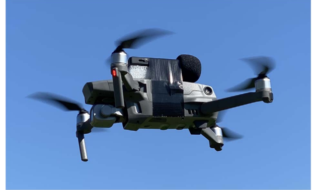
Figure 8. On-board recorder mounted on top of a DJI Mavic 2 Pro.
