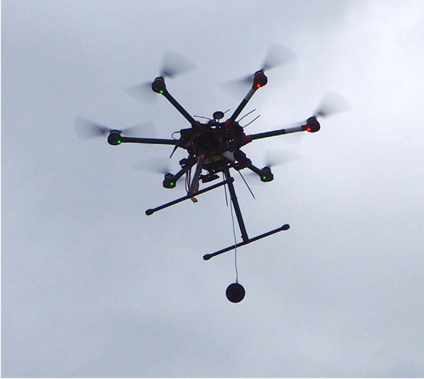
Figure 7. On-board microphone attached to the flying drone.
