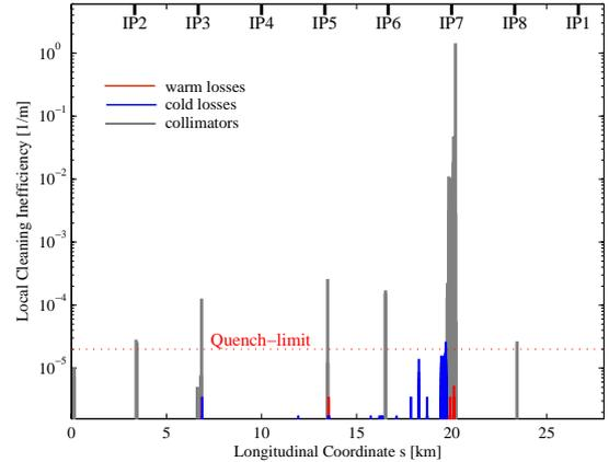
Figure 1: Proton loss map for Beam 2 betatron cleaning at 7 TeV (horizontal halo). The full phase 1 collimation system is simulated with collision optics. Blue bars correspond to losses on SC elements, red bars to losses in warm elements and grey bars to inelastic interactions in collimators. The beam moves from the right to the left. The estimated quench limit refers to nominal intensity ( $3.2 \times 10^{14}$  protons) and 0.2 hours beam lifetime.
