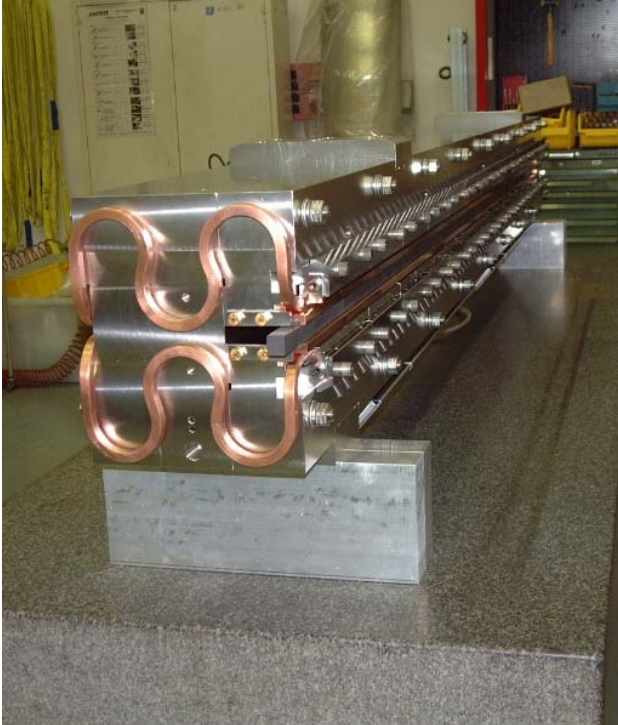
Figure 4: The new TPSG4 diluter in its yoke, before installation in the vacuum vessel.
